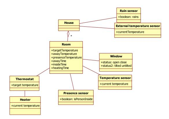
A house has several rooms, a rain sensor (tells if it rains or not) and an external temperature sensor (reads temperature outside). A room has a heater (radiates heat from water to air) controlled through a thermostat (open closes a valve that controls water intake in the radiator, trying to keep a set target temperature), a window (can be open closed, or tilted), a presence sensor (tells if a person is inside or not), a temperature sensor (reads the current temperature in the room).
