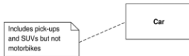
A note is used as a comment on one or more diagram elements
